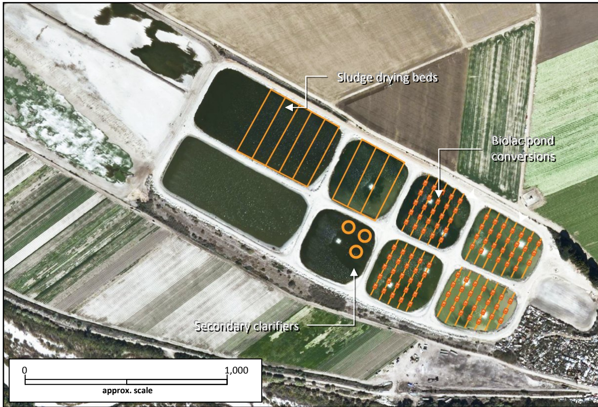
Figure 5.3: Estimated area required for an expanded facultative pond treatment system at buildout.
